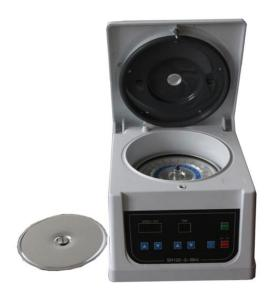
Microhematocrit Centrifuge is used for accurate determination of blood cell and also for precipitation and separation of little amount blood and solution. Take a little amount of blood, (you can use the blood of ear-lap which is convenient to get) which can be centrifuged in a very short time. It has the merits such as high work efficiency, integrated design and high accuracy.
